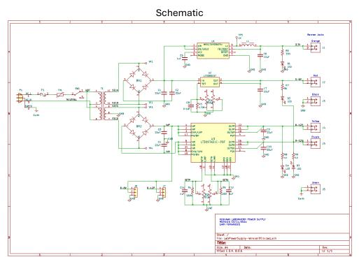
The board is the physical realization of the schematic, with component footprints positioned on the board and copper tracks making the connections described in the schematic. Footprints are a set of copper pads that match the pins on a physical component. When the board is manufactured and assembled, the component will be soldered onto its corresponding footprint on the circuit board.
